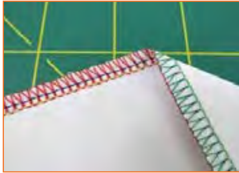
Fig 2.2.8(b): Five-Thread Overlock
