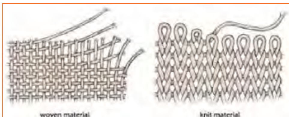
Fig 2.1.2: Difference of Woven and Knit material
