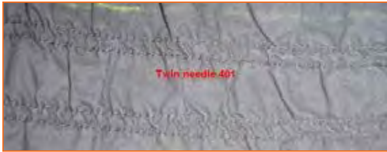
Fig 3.2.9: : Shrinkage pucker occurs during the
