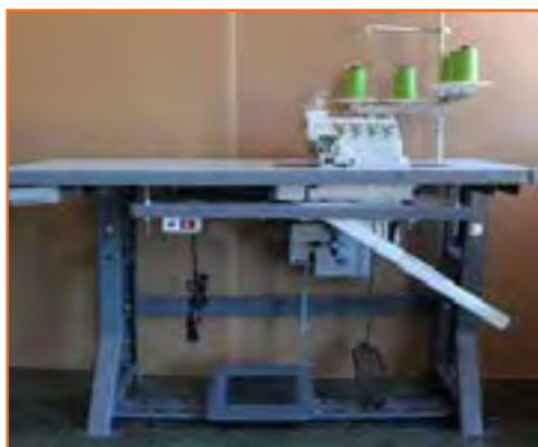
Fig 2.2.7: Four Thread Overlock Machine
